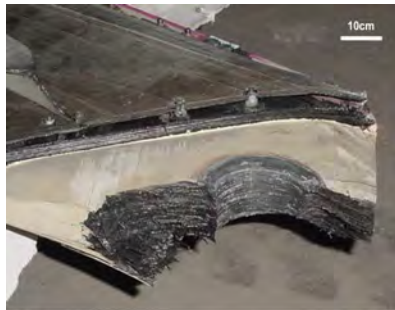
Lug failure from A300 Airbus tail (2001)
